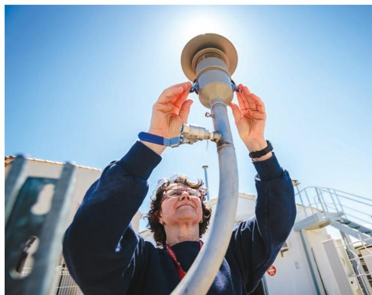
PRÉLÈVEMENT D'UN FILTRE PAPIER PIÈGEANT LES AÉROSOLS DE L'AIR
